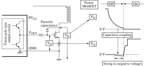
Figure 8. V<sub>OUT</sub> terminal description
