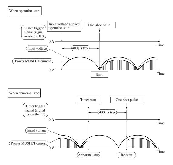
Figure 9. Explanation of timer operation
