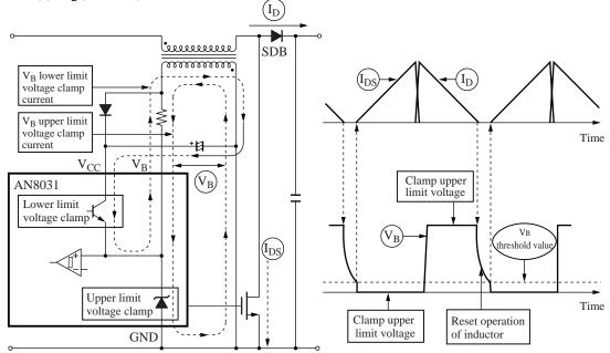
Figure 5. Explanation of  $V_B$  operation
