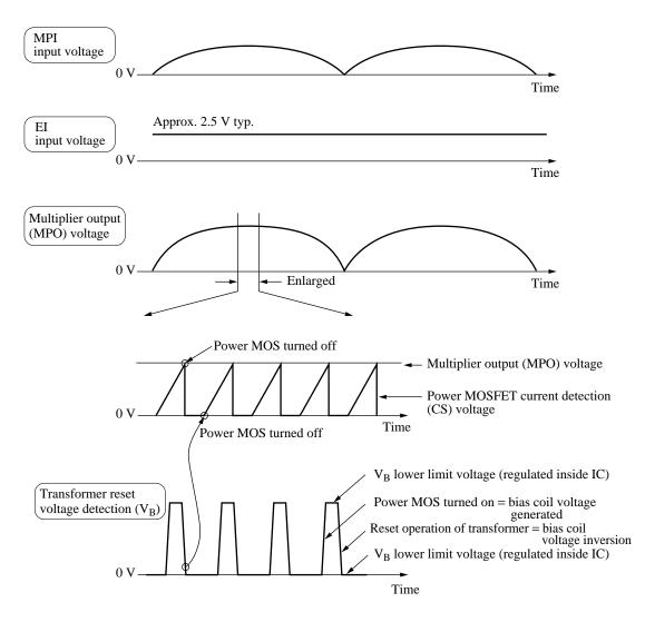
Figure 2. Explanation of normal control operation
