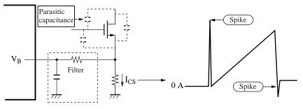
Figure 6. CS terminal explanation
