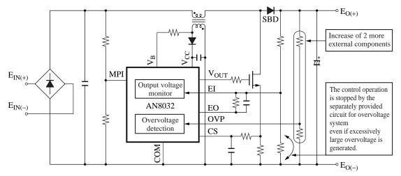
Note) The OVP terminal is arranged beside the EI terminal after taking the board pattern design into consideration.
