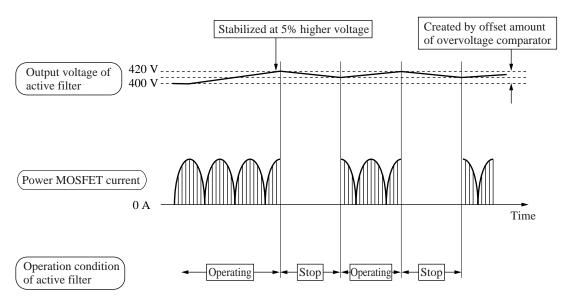
Figure 11. Protection of overvoltage protection operation
